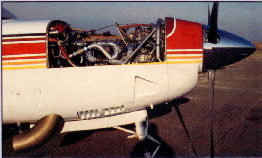
One concern that must be carefully handled is that turbine exhaust fumes might enter the cabin either on the ground or in flight. The exhaust stacks on the Garrett TPE331 (shown . . .
