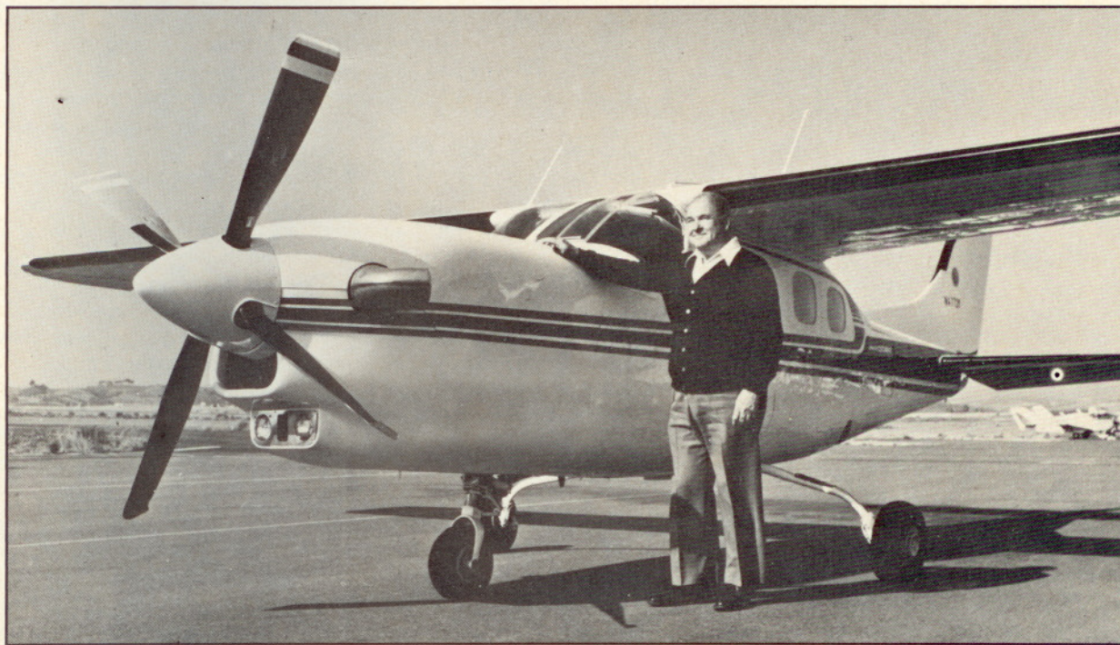
Jack M. Riley, president of Riley Aircraft Manufacturing, stands by the prototype P210 turbine conversion. The cowl has been redesigned since this photo was taken, and the craft should receive a three-blade propeller, changes that are expected to improve performance.
